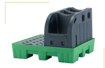
Ref. 9217W04 Comprising the spill control 9215W04 and drum holder 8961004 240 litres Ext. Dim. : L 1300 x W 1300 x H 285 Static load: 1600 Kg. Weight: 72 Kg.
